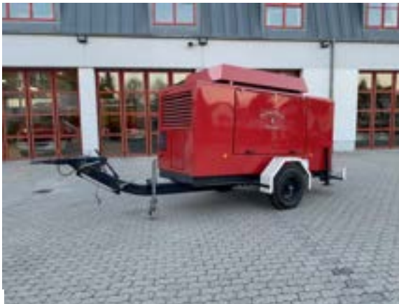
Notstromaggregat 86 kVA Bosch (1989)
